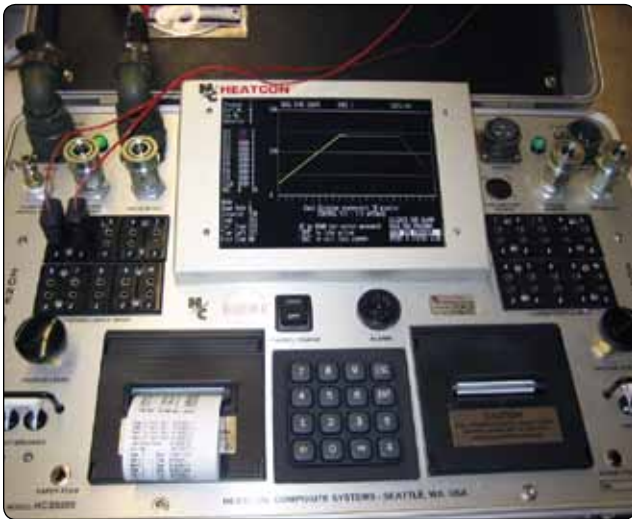
Figure 7-40. Heat bonder equipment.
