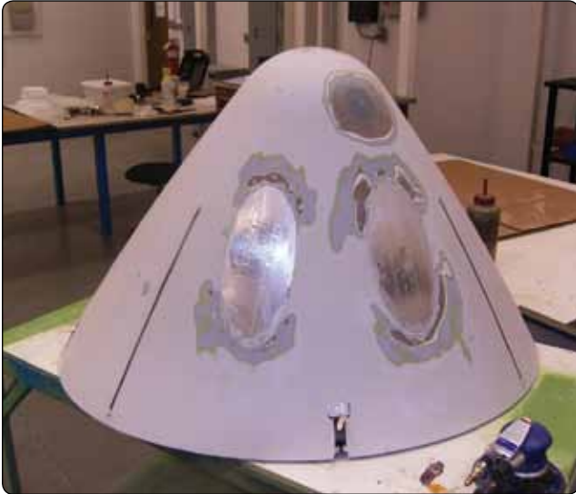
Figure 7-21. Damage to radome honeycomb sandwich structure.
