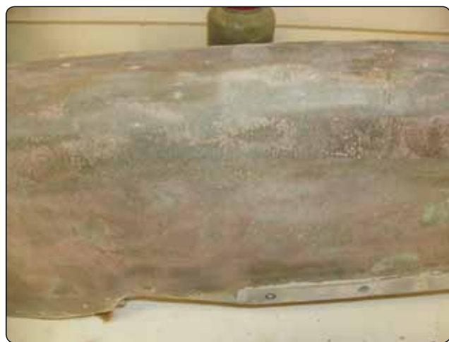
Figure 7-8. Copper mesh lightning protection material.
