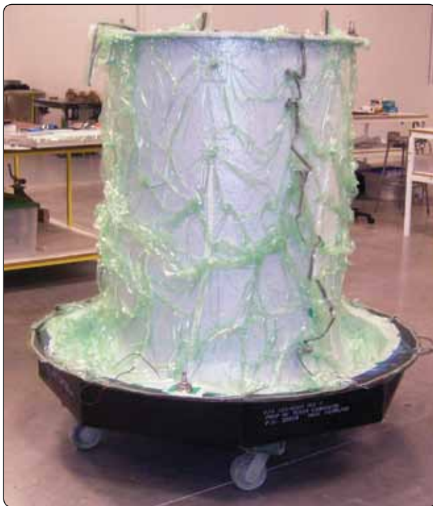
Figure 7-36. Bagging of complex part.
