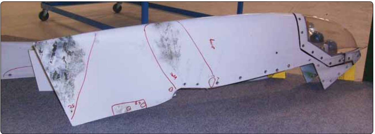
Figure 7-22. Erosion damage to wingtip.
